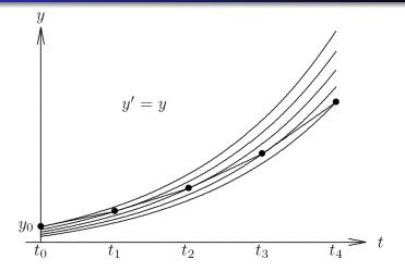
For unstable solutions, errors in numerical solution grow with time
